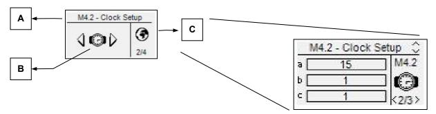
Press "i" to confirm and enter, or press the left or right arrows to see the next submenu, or press "menu" to return to the previous screen. In the submenus, the parameters are divided in different pages; choose the page with the left and right arrows, and choose the parameter with the up and down arrows. Then press "i" to confirm and modify the parameter. Then press "i" to confirm or "menu" to cancel.
