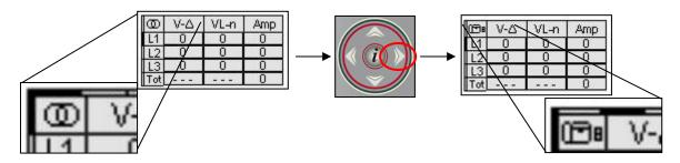
• The cursors on the upper side and left side of the display indicate the position of the page inside the navigation diagram: the left and right arrows move the page along with horizontal cursor.
